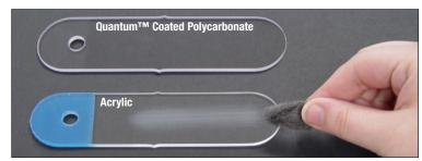
We use a steel wool scratch test to demonstrate the abrasion resistance of Quantum coated polycarbonate (top) against acrylic (bottom).
