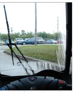
Award-winning Quantum coating is used in many tough applications. Our Quantum coated polycarbonate has withstood over one million windshield wipes on the windshield of the fully enclosed Benelli Adiva scooter.
